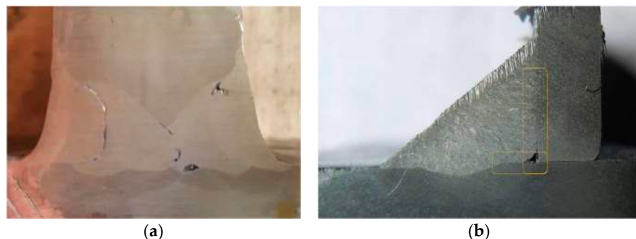
Figure 7. (a) Lack of fusion due to improper handling of the gun, applying the arc heat unevenly; (b) incomplete fusion as a result of the weld pool being ahead of the electric arc, preventing proper fusion.
