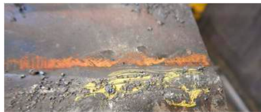
Figure 6. Spatter produced by the use of inadequate wire feed rate.
